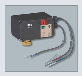
TROVIS 5724-8/5725-8 - They are the allrounders among the electric actuators with process controllers and can considerably reduce the energy consumption in heating and cooling applications. Fixed set point, follow-up, override or cascade control can easily be implemented using preconfigured plant schemes. The set points and operating mode can conveniently be adjusted on the control panel on site. Devices with RS-485 interface can be connected to the SAM DISTRICT ENERGY interface.
