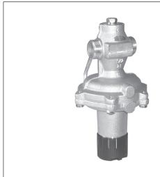
Fig. 1: Type 45-6 Differential Pressure Regulator, DN 20 · With rotary knob and scale division · Set point range 0.1 to 1 bar
