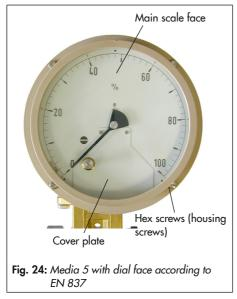
This allows, for example customized dials for filling level measurement to be calculated based on the tank geometry data.
