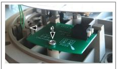
Fig. 19: Inserting the terminal board
