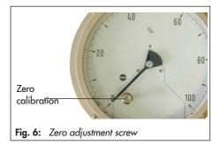
As a result, errors caused by the mounting position or static pressure are eliminated.
