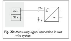
The option module consists of an actively controlled current loop with a 4 to 20 mA loop current. This current depends on the position of the pointer on the Media 5 device:
