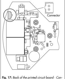
ig. 17: Back of the printed circuit board · Connector for the terminal board
