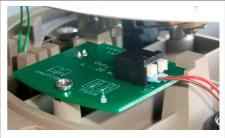
Fig. 21: Connecting the measuring signal lines on the terminal board
