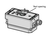
Fig. 5-1: Vent opening (back of the positioner)
