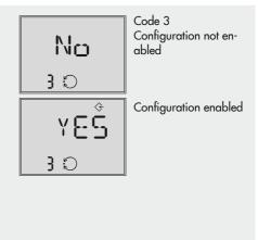
If no settings are entered within 120 seconds, the enabled configuration function becomes invalid and the display returns to Code 0.
