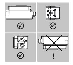
Fig. 5-2: Permissible mounting positions
