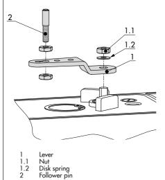
Fig. 5-4: Mounting the lever and follower pin
