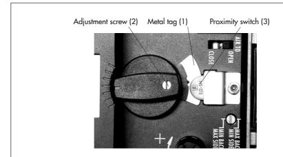
Fig. 7-4: Adjusting the limit switch
