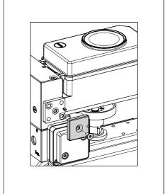
Fig. 5-14: Mounting the turnboard
