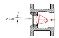
As a result, open the valve slightly (angle of approx. 2° to 3°) before start-up and close it again after start-up when the process medium has distributed the heat evenly (see drawing).
