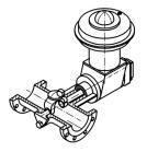
The actuator must be installed in vertical position. Mounting the actuator in a different position can lead to defects and thus malfunctions.
